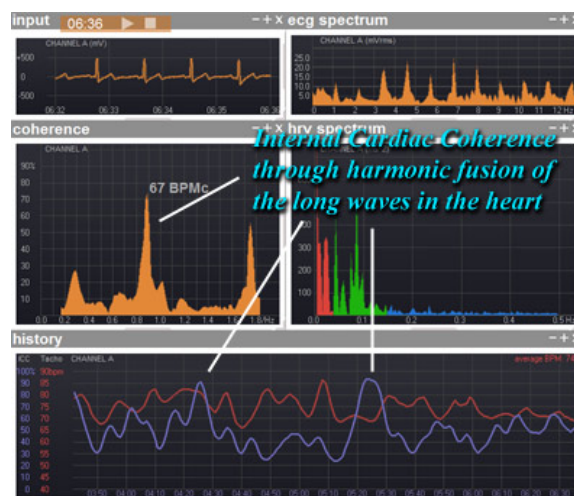
CardioGem - Internal Coherence diagnostic and biofeedback program, showing respectively: raw data ECG, ECG Spectrum, Internal Cardiac Coherence (ICC), Heart Rate Variability (HRV) Spectrum, Tachogram (Beats Per Minute) and ICC history (statistics and other evaluation tools and biofeedback environment not shown here).
