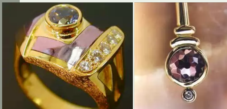
The addition of aluminum to gold creates a brittle purple gold. Purple gold used in a pin, and a purple gold inlay within a yellow gold ring.
