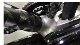
3D-printed titanium offers new possibilities for bike builders
